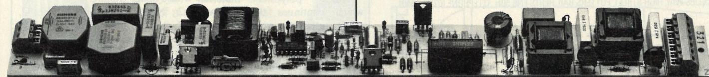
This is because the WOTAN QUICKTRONIC® DE LUXE is fully electronic and operates at high frequency. As a result, lamps start without flicker in only 0.1 second. They continue to work free of flicker and hum, and without stroboscopic effects or radio interference. There is also a reduction in heat generation.
